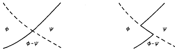
Figure 1. Possible fragments on the phase diagram of the system. The full curves represent the first-order phase transition, the broken ones those of second order.
